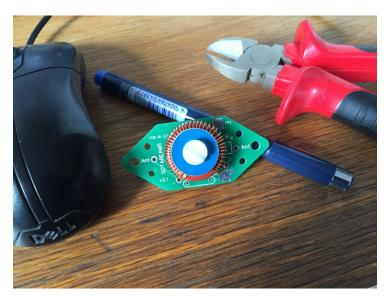
Prototype 7 MHz trap using a SOTABEAMS trap PCB
