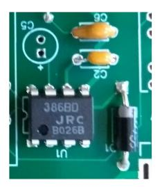
Install the diode, ensuring that it is fitted the right way round.
