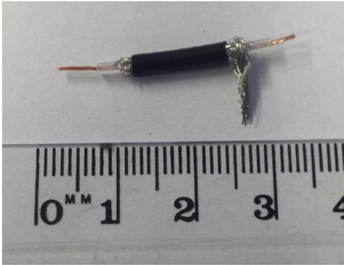
7. Install the coaxial cable coupling lines through the toroids on the board as shown. Note that the braid is soldered to the pad that has a number of plated-through holes on it.
