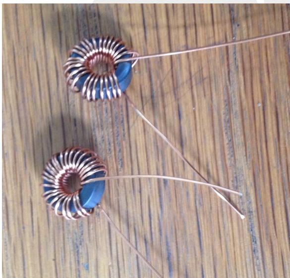
3. Tin the leads for the cores and solder the core into the marked positions on the board (T1 and T2). Note the cores sit vertically.
