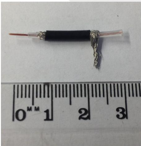
6. Remove 5mm of the inner insulation and tin the exposed centre core of the co-axial cable.
