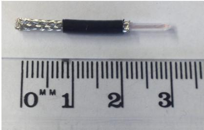
7. On the end where you have trimmed the braid, remove 5mm of the inner insulation and tin the exposed centre core of the co-axial cable.
