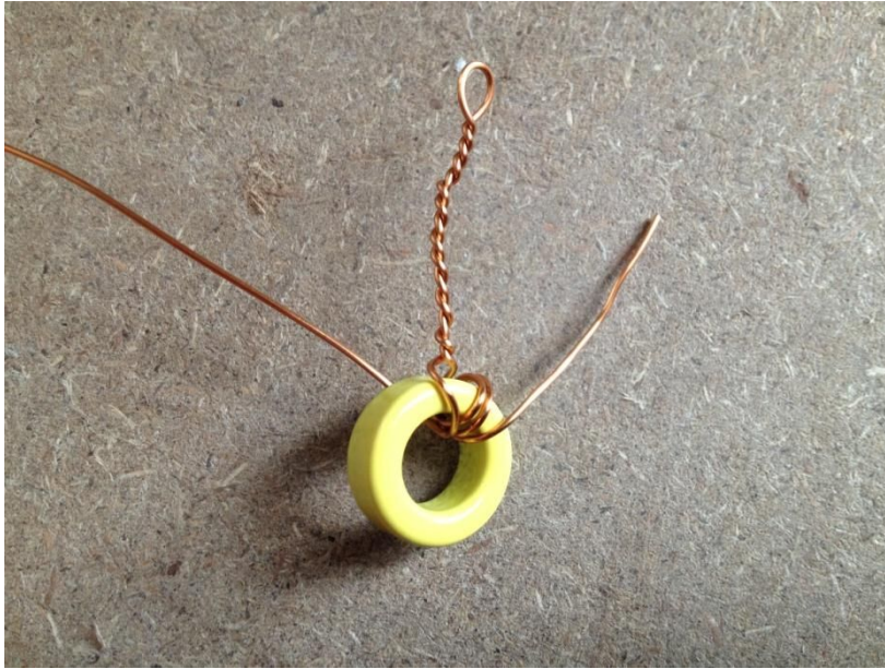
Photo shows 3 turns, the twisted tap and a fourth turn.
