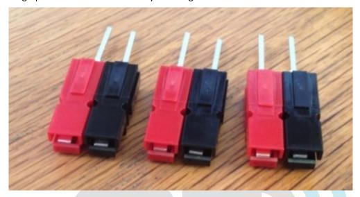
3. Insert the pairs into the PCB. Make sure that they are all the same way round and that the red shell is in the positive position as marked on the PCB.
