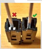
2. Pair up, the shells as shown, one black and one red. Slide the red along the black to lock the two together.
