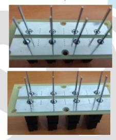
Bridging the track spokes is not a problem – it reduces the resistance. The spokes are there to help you get the board/pins up to temperature for soldering.
