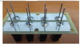
6. Cut the surplus parts of the pins off – do not close-crop them – leave the solder intact.
