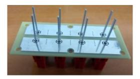
5. Solder one of the pair of pins check the shell is flush with the board. If not reheat the solder and push the shell flush with the PCB. Solder the other pin.
