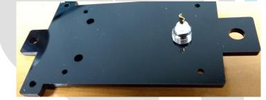
On the rear of the panel. The serrated washer goes on first, then the solder tag and finally the nut. Do not over tighten the nut as you could crack the front panel.
