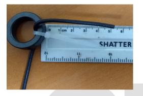
□ Wind a further six turns then thread through the centre to the other side as shown in the figure below (this figure shows 4 turns on one side and 3 turns on the other).
