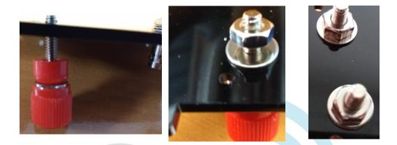
Top Tip:- Unscrew the plastic tops of the binding posts a few turn before tightening the nut. Tighten the nut whilst holding the plastic post closest to the panel. Do not over tighten, otherwise the panel may crack.
