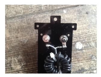
□ Solder the other end of the coaxial cable to the BNC socket as shown.
