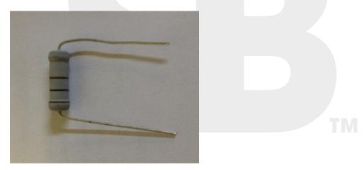
3. Lay the plastic spacer on the **top** surface of the printed circuit board (pcb) and install the resistors (R10 and R7) as shown. Make sure that the resistors are in contact with the spacer. Hint – for a professional look, mount them all the same way round.
