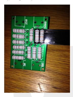
This completes installation of the load resistors.
