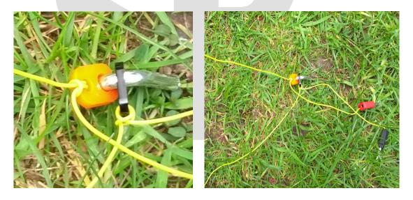
Plug the black banana plug on the end of the radial into the black socket on the adapter. Plug the red banana plug into the red socket on the adapter. Connect the adapter to your radio.
