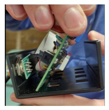
Unplug the ribbon cable, then pull the black cable through the grommet to allow the PCB to be worked on.
