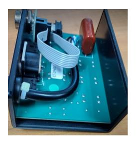
Removing the PCB
