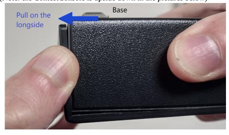
The bottom half should then slide out of the top half.
