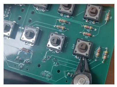
On the switch side nearest the resistors, use the cutters vertically to cut the legs.
