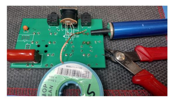
When the holes are clear of solder, fit and solder the new switch.
