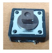
Remove the legs from the PCB. Solder suckers and/or desoldering braid are useful for this.
