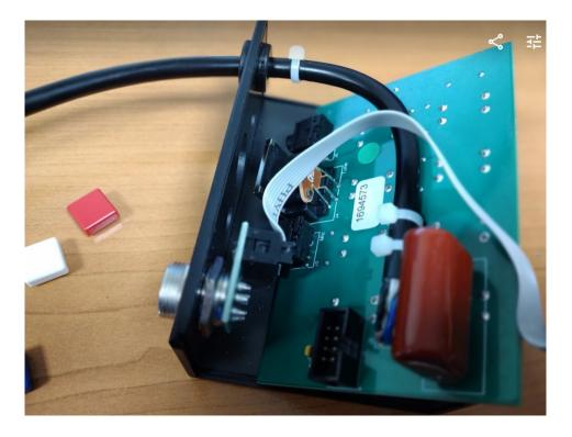
Rotate the PCB under the side connections and push down until it clicks into place.
