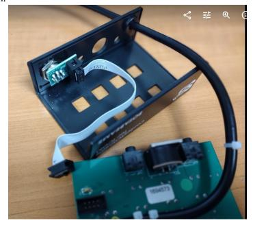
Remove the switch caps by pulling the cap up. Removing all the caps will make it easier to refit the PCB into the case.
