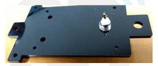
On the rear of the panel. The serrated washer goes on first, then the solder tag and finally the nut. Do not over tighten the nut as you could crack the front panel.
