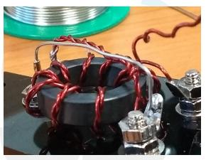
Wire **a** is soldered to the same tag. Remove enamel from wire a, and twist it around the tinned copper wire (trim to length). Tin the twisted wires and solder to the black post solder tag.
