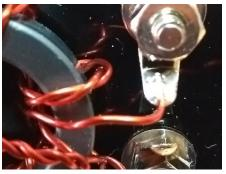
☐ Bend the tinned copper wire to run parallel to wires **A,b** Bend the wire down to the black solder tag, cut to length.
