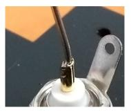
☐ Tin the two post solder tags and BNC solder tag.
