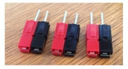
7. Insert the pairs into the PCB. Make sure that they are all the same way round and that the red shell is in the positive position as marked on the PCB.
