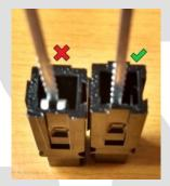
6. Pair up, the shells as shown, one black and one red. Slide the red along the black to lock the two together.
