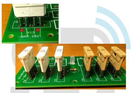
Invert the PCB onto a flat firm surface. Check that all the fuses are all straight.
