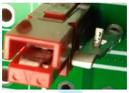
Ensure the pin is fully engaged. This can be felt as two clicks if pushing gently. Note that you may need to move the pliers back a bit to get the second click.
