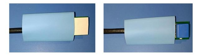
Heat the sleeving until it is gripping all four corners of the PCB, ensuring that it is tight over the resistors, wires and cable ties.
