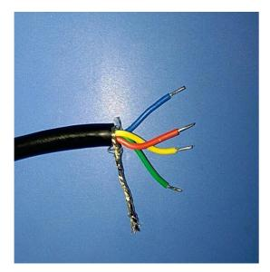
Push the corresponding wires through the holes on the PCB and solder them in place. (1=Red, 2=Yellow, 3=Blue, 4=Green)
