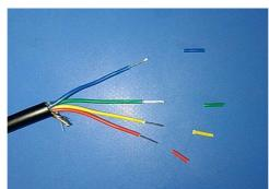
Remove the cotton and plastic as before. Trim the braid to 5mm and strip the rest of the wires by 1cm.
