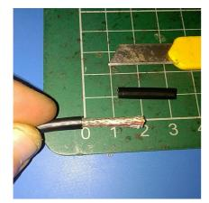
Push the braid back and pick the strands apart using a small screwdriver or tweezers. Separate the braid into two pieces either side of the wires and then twist the two parts together as shown below.
