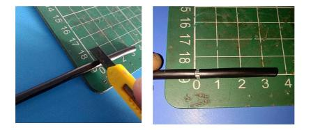
This task requires something small and pointed; I would recommend a small flat-headed screwdriver or tweezers. Push the braid back on itself and separate the small strands. You should then twist the braid as shown below. (This is the same process as used in the PCB assembly)
