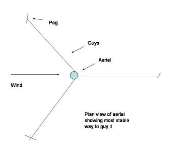
At the other end of each cord, tie a simple slip knot. To use the guys, slide them over the aerial, tighten the slip knot and peg. Always try to attach the guys to a point above the top plastic connecting sleeve or above the plastic T-piece (whichever is higher).
