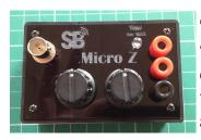
Thank you for purchasing a Micro Z (pronounced "Micro zee") antenna tuner. The Micro Z has been designed to provide a wide matching range across the 7 to 28MHz frequency range (40m-10m). Like any tuner, the precise range will depend on the antenna that you are tuning.
