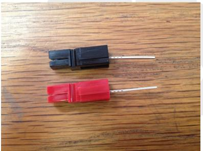
2. Pair up, the shells as shown, one black and one red. The shells will pair up in many ways so make sure that you get them right – as shown in the photograph. This is the "standard way" of using Powerpole connectors for ham radio use.
