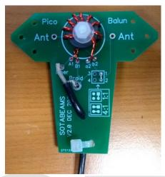
☐ If using RG58, lay it against the PCB.
