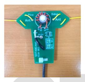
The Pico Balun can be mounted to a fibreglass mast using our <u>Versatile Top Antenna</u> <u>Insulator</u> and cord.
