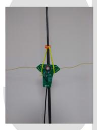
Your Pico Balun will need to be protected from rain. You can coat it with our <u>Liquid Electrical Tape</u> which does not affect the operation of the circuit (once fully dry). Some other sealants will reduce the Q of the circuit and the acid solvents used may corrode the exposed wire and PCB pads – beware.
