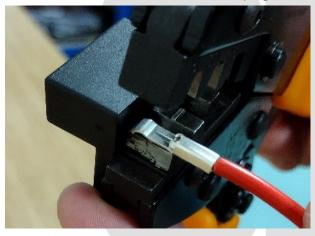
Ensure the shoulder of the contact is flush with the back plate of the tool.
