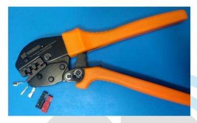
Insert the wire and contact into the crimping tool. Ensure the crimp is not upside down
