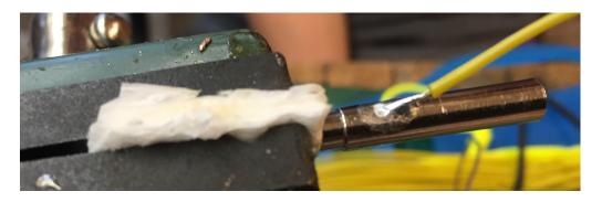
4. After letting the body of the plug cool completely; insert it into the shell as shown and snap the shell closed.
