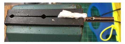
2. Tin the hole, being careful not to overfill as the solder will flow through the plug.
