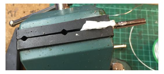
3. Tin the wire and solder into the hole in the plug body.
