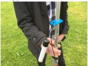
The antenna can be attached to a pole using the attachment fitting supplied.
