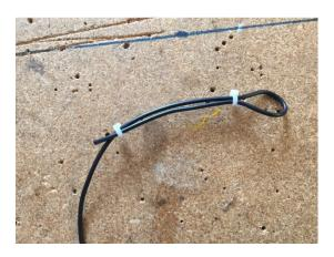
Adjusting the 20m/10m section of the antenna is not generally recommended as it will change the resonant frequency on 20m, 10m and 40m.
