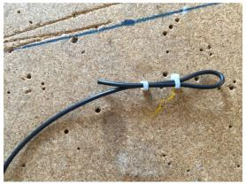
Fold back the antenna along itself. If the cable ties are not too tight you can easily slide the wire back to change the resonant frequency.
