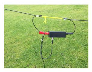
The matching network sits below the antenna. The red plug (antenna) fits in the red socket and the black plug (counterpoise) in the black socket. Note how the feeder strain-relief loop is attached.
